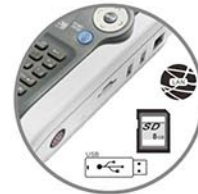
Peripheral ports: SD card, USB, LAN
