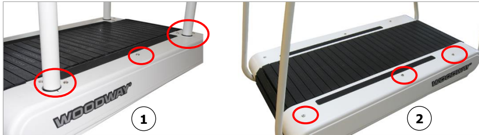
Fig. 22 Side panel fixing screws
