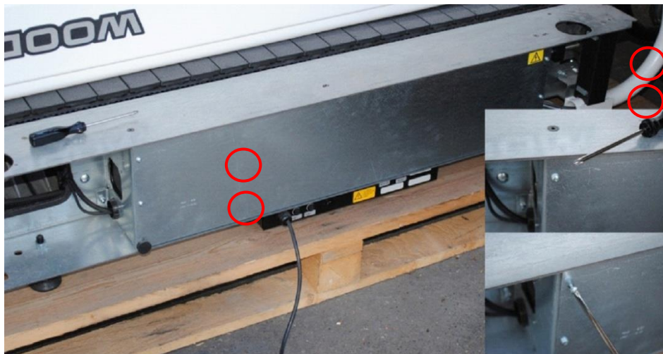
Fig. 23 Remove electronics shielding panel
