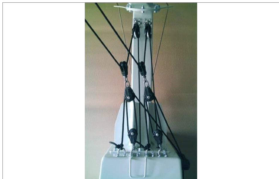
Fig. 26 ELVETA, Two-Sided Rope Length Adjustment
